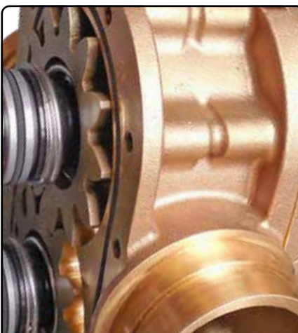
Bronze Pump Rotors and Mechanical Seals
